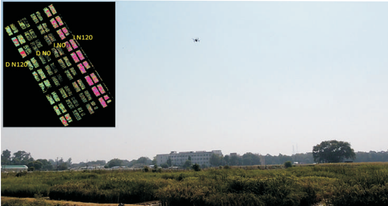
Figure 1. Use of drones for phenotyping. Inset shows image obtained from the Drone clearly distinguishing crop with different irrigation and nitrogen treatments.
