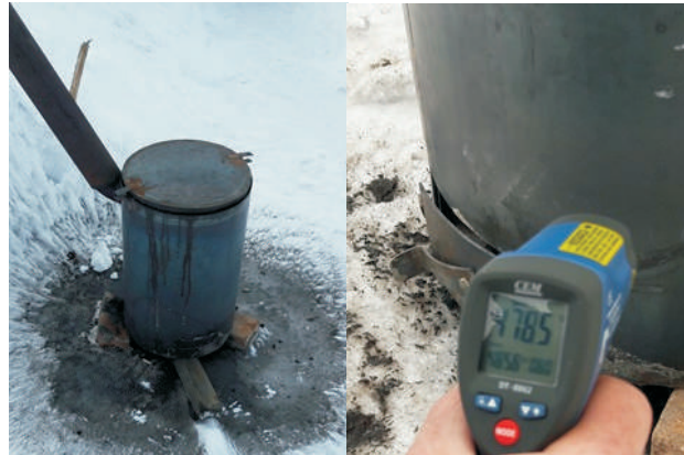
The oven is at work. The temperature reaches 550 degrees centigrade
